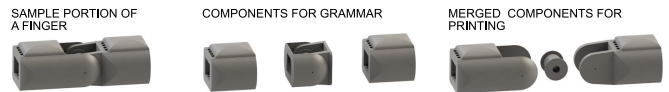
Fig. 6. Grammar components correspond to mechanical systems rather than physical parts. They can be combined into their proper physical parts that are suitable for 3D printing after deformation.
