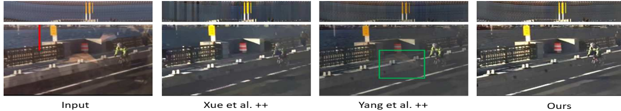
Figure 10. Our removal against advanced video extensions of the state of the art (‘+’ and ‘++’). Yang et al. ++ generates incomplete separation (see green box) while Xue et al. ++ blurs the cyclist, the sea and generate temporally incoherent results (see the red slice). Our approach significantly reduces temporal flickering, image blurriness and improves separation.
