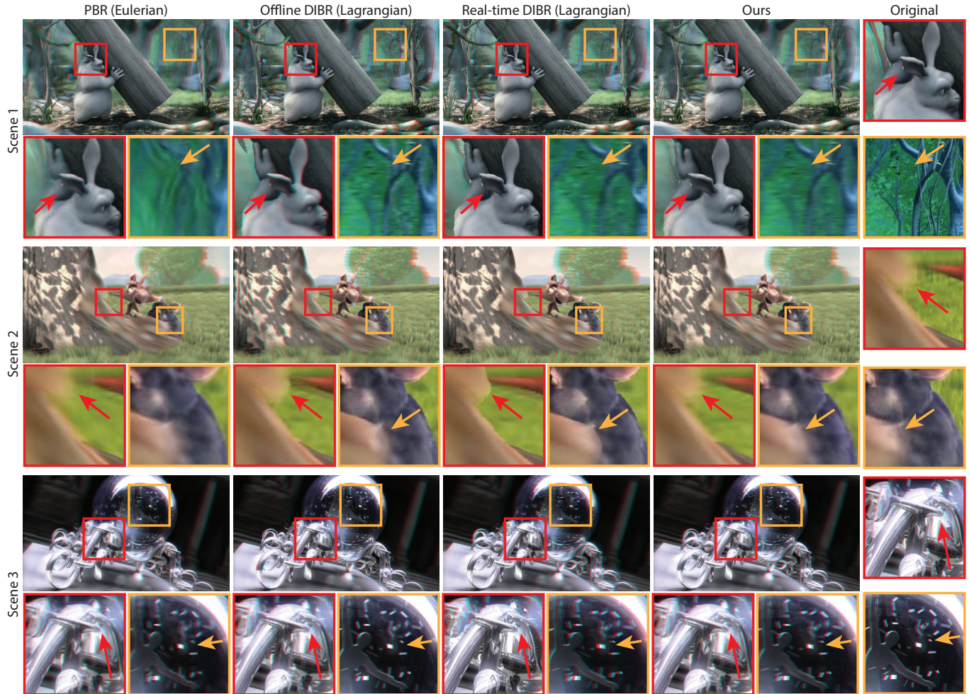
Fig. 7. Columns: Comparison of the same red-cyan anaglyph stereoscopic views produced by PBR, offline full-resolution DIBR, real-time DIBR and our algorithm as presented to participants in our user study. Rows: “Big Buck Bunny” © by Blender Foundation (Scene 1 and 2) and “Ball” © by Eric Deren / Dzignlight Studios (Scene 3).
