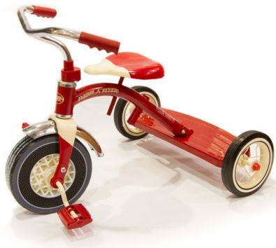
Figure 13. The tweel mounted on a toddler tricycle.
