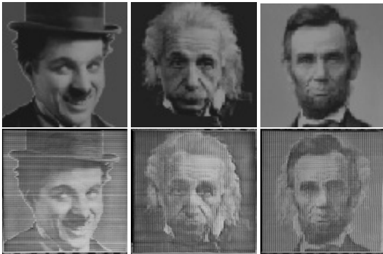
Figure 10: Input images (top row) and photographs of a single SHADOWPIX produced by the local method (bottom row).
