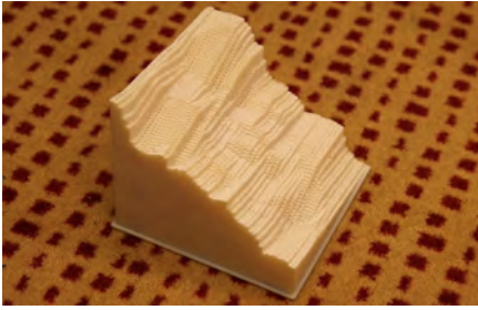
Figure 5: Without chamfering, the local method produces SHADOWPIX that are too tall to be usable. The height increase is necessary to prevent a part of the surface closer to the +y light direction from shadowing a part of the surface farther from the light direction (see Equation (3)). Chamfering produces SHADOWPIX whose maximum height is about 1 cm for an image that is 20 cm on each side.
