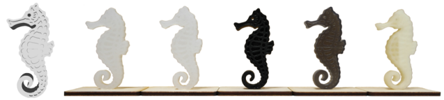
Figure 13: From left to right: a rendering of the original seahorse model. Seahorse models used for the study: Dragon Skin 30, Ecoflex 00-30, TangoBlack+, Flexible resin, TPU 92A-1.
